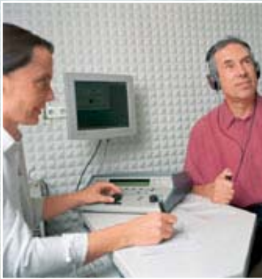
Scientists researching human hearing have determined that most people perceive a 10 dB increase in sound energy over a given frequency range as roughly a doubling of the loudness.
