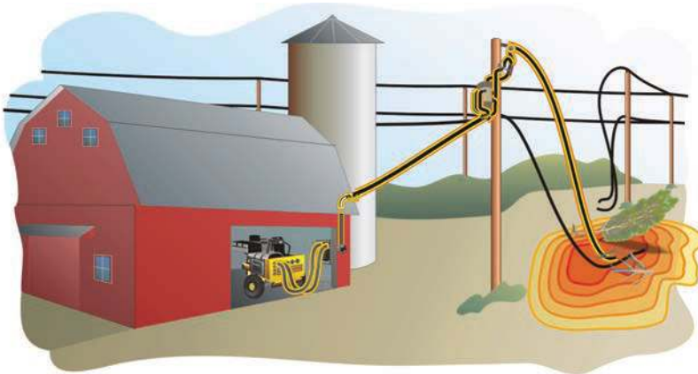
Backfeed from Generator
