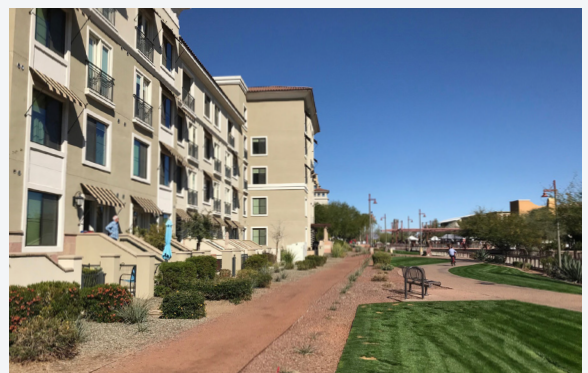
Connect public space and private space utilizing a clearly defined transition between the two. The residential development shown above utilizes a low, transparent wall and plant material to distinguish the boundary between public and private areas.
