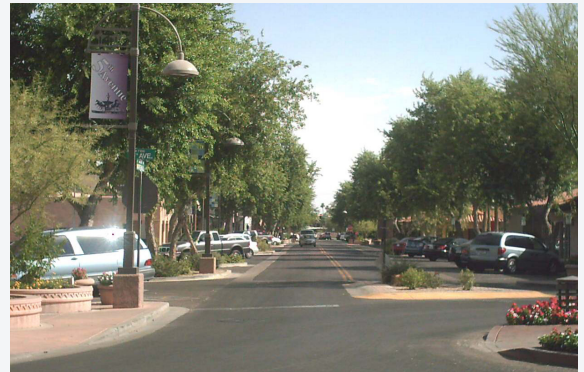
Consistent building setbacks, and a streetscape featuring linear and rhythmic tree plantings, provide street-space continuity.
