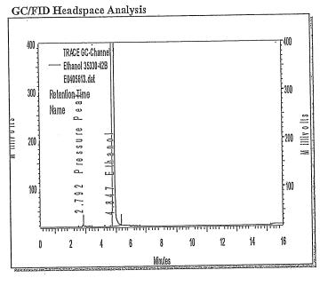
DB-ALC1 30 m x 0.53 mm, 3  $\mu m$  film thickness Column: 40°C (12 min) to 220°C at 40°C/min (5.5 min) Temp Program: Helium Carrier Gas:
