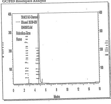
DB-ALC1 30 m x 0.53 mm, 3 µm film thickness Column: 40°C (12 min) to 220°C at 40°C/min (5.5 min) Temp Program:
