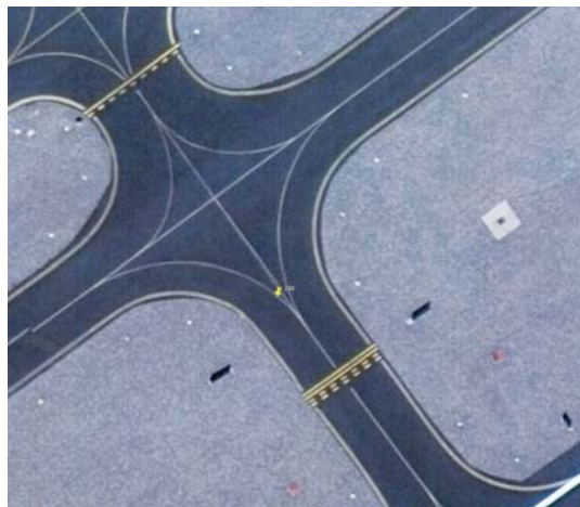
Figure 4 – Revised Hold-Line Relocation
