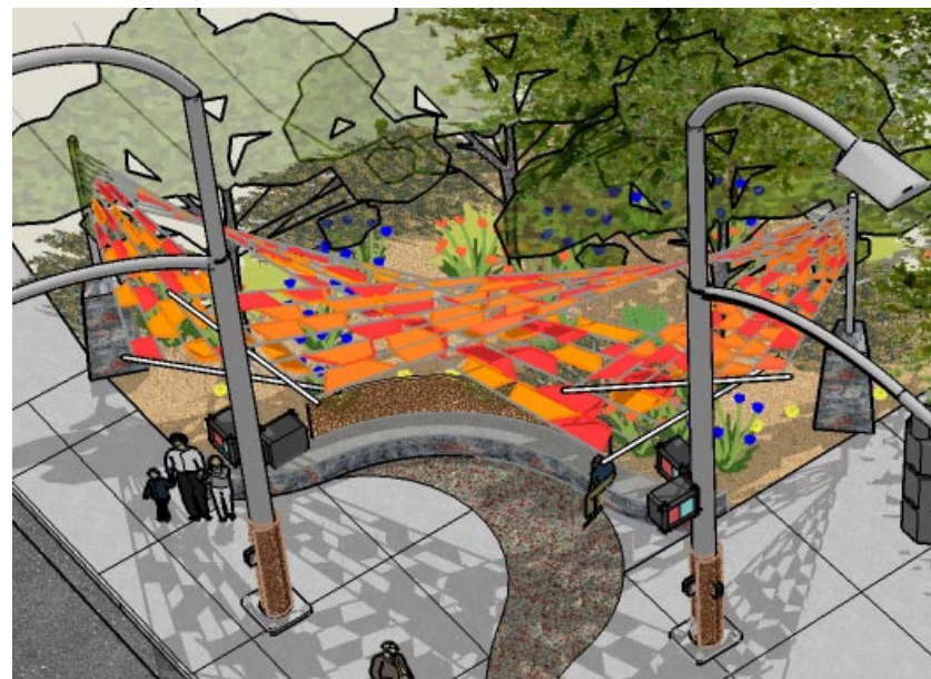
Dry laid sandstone pier with trapezoid shape low walls and metal seat backs at primary Green Spots
