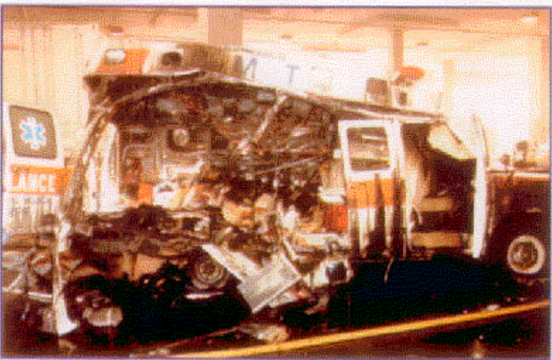
Extensive fire and structural damage to the ambulance unit. (CS1-8)
