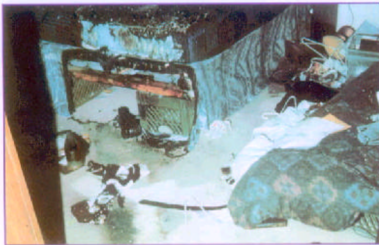
Obvious pour patterns extend from the bed where the occupant was sleeping at the time of the arson. (CS6-4)
