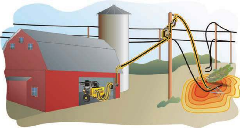
Backfeed from Generator
